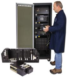
PSI's functional test system simulates down-tower and up-tower communication and component interface. PSI can also identify and correct "watch dog" errors.
